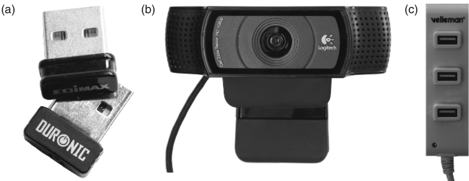
Figure 1-10: (a) USB Wi-Fi adapters; (b) the Logitech C920 camera; (c) a Velleman USB hub (bus powered)
