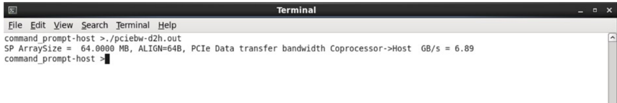
Figure 6-4. Output of the PCIe BW-d2h test with 64MB data read with 64B alignment
