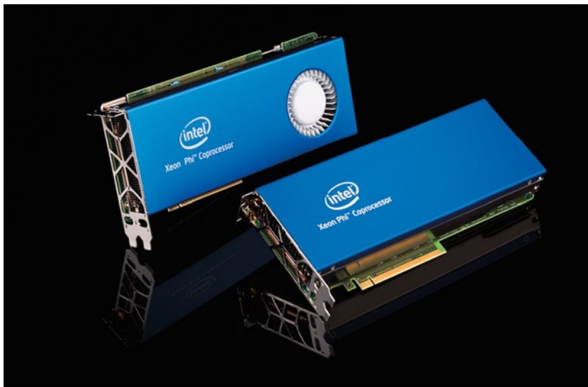
Figure 1-10. Intel Xeon Phi coprocessors in actively-cooled and passively-cooled versions. (Source: http://newsroom.intel.com/docs/DOC-3126#multimedia )
