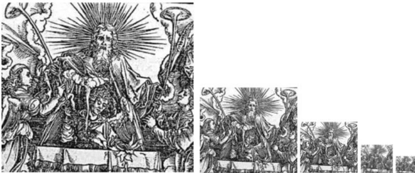
Figure 4-16. A five-octave scale pyramid. The image is from Albrecht Durer's Apocalypse woodcuts, 1498. Note that many methods use non-octave pyramid scales [120]
