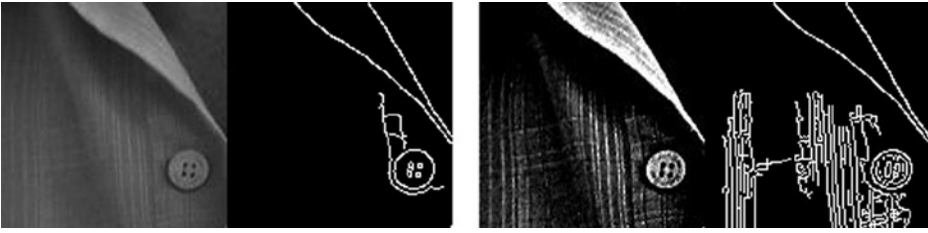
Figure 2-2. The effects of local contrast on gradients and edge detection: (Left) Original image and Sobel edges. (Right) Contrasted adjusted image to amplify local region details and resulting Sobel edges
