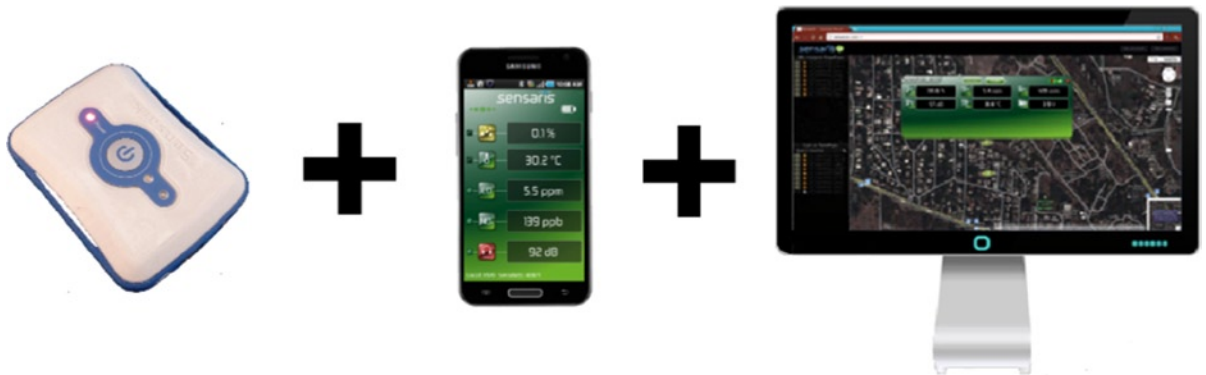
Figure 11-8. The Sensaris SensPods system for mobile ambient environmental monitoring (image used with permission from Sensaris - www.sensaris.com )
