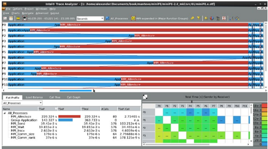
Figure 5-7. MiniFE trace file in ITAC zoomed in upon the offending MPI_Allreduce operation (Workstation, 16 MPI processes)
