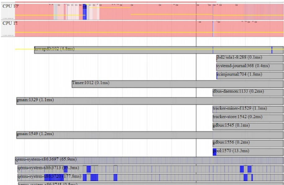
Figure 7-17. Timechart part 2: software thread activity
