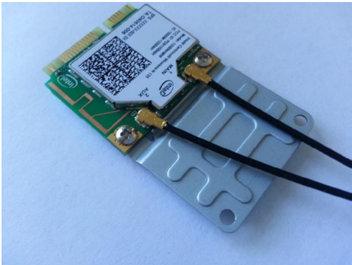
Figure 5-2. Antennas connected to the WiFi card
