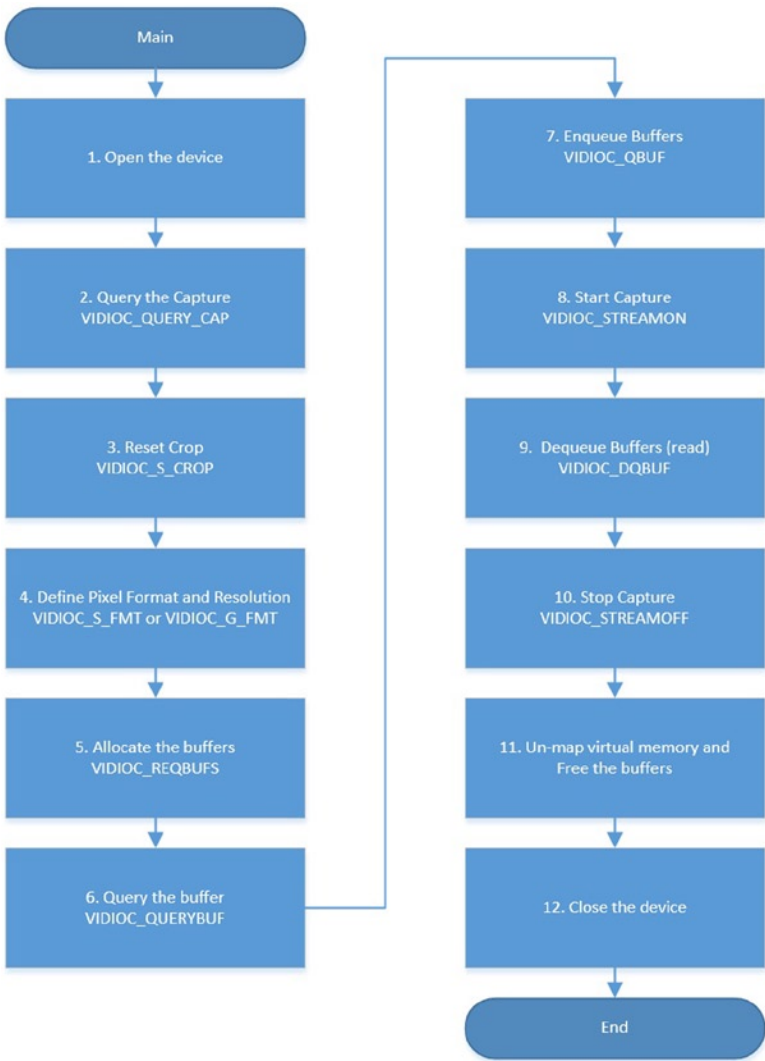
Figure 7-4. Flowchart related to capturing video using V4L2
