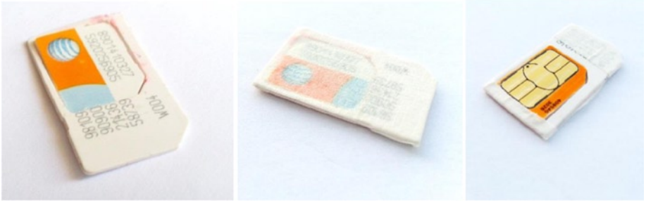
Figure 12-4. Inserting the nano-SIM and taping it to the adaptor
