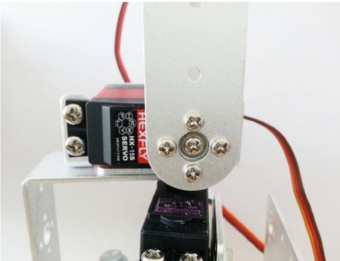
Figure 11-22. Connecting the shoulder servo and the U-shapes
