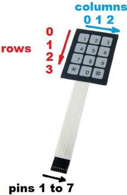
Figure 9-4. Keypad disposition of pins and identification of rows and columns
