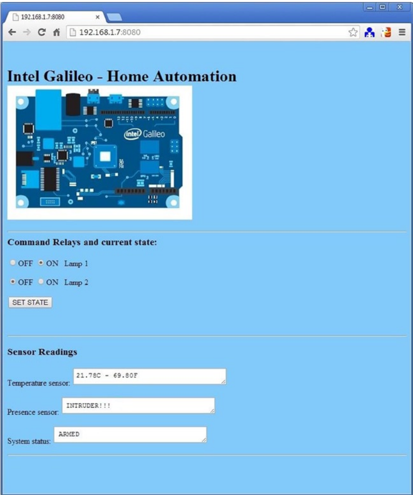
Figure 9-20. Dynamic web page is working
