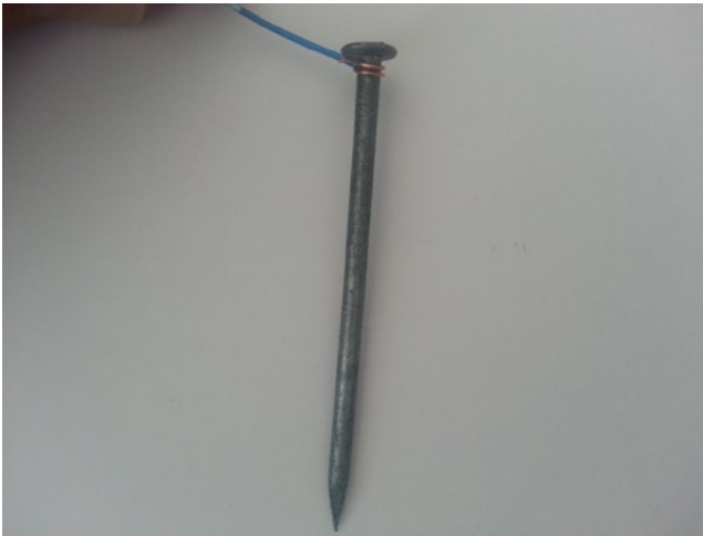
Figure 8-4. Wrapping the wire around the nail's head
