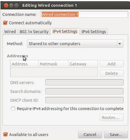
Figure 5-13. IPv4 Settings sharing the Internet
