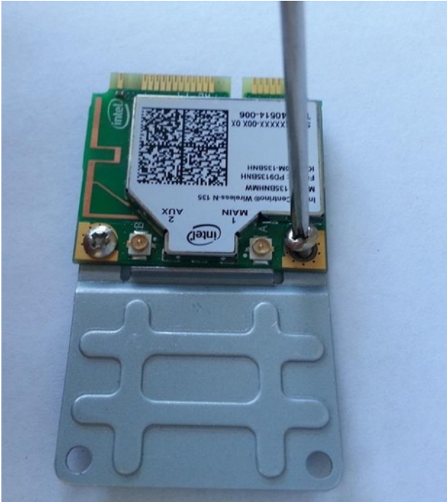
Figure 5-1. Connecting the bracket to the WiFi card
