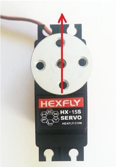
Figure 11-12. Servo wheel placed at 90 degrees
