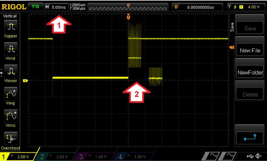
Figure 4-10. When pinMode() takes 3ms to change the port direction
