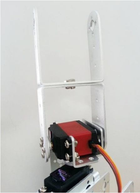
Figure 11-23. Connecting the shoulder servo to the arm
