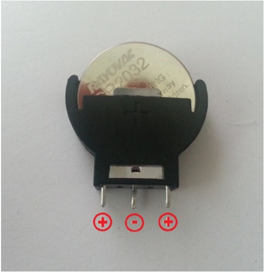
Figure 6-2. Coin battery 2032 in the case and the polarity
