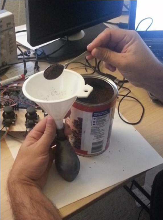
Figure 11-51. Filling the gripper with ground coffee
