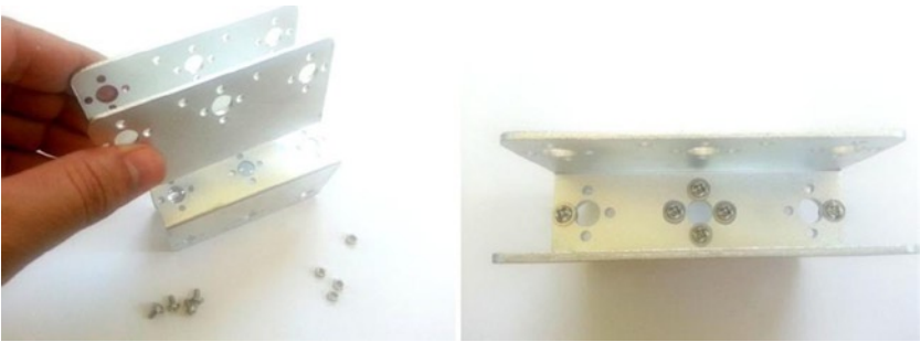
Figure 11-13. Connecting two U-shapes for the base
