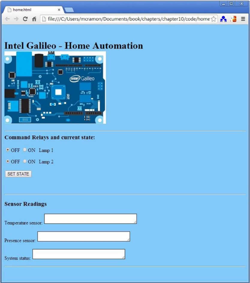
Figure 9-18. Web page design for home automation
