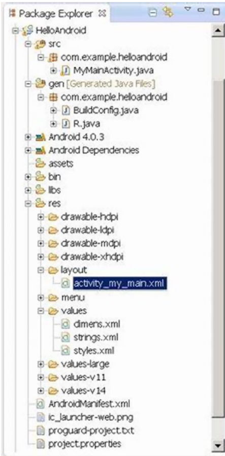
Figure 7-4. Example file structure of an Android project
