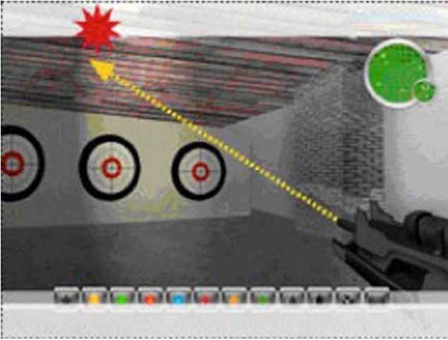
Figure 1-3. Screen-mapping errors due to a high aspect ratio
