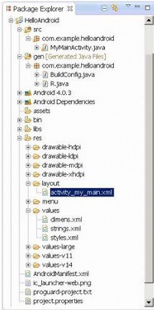
Figure 1-4. Example file structure of an Android project
