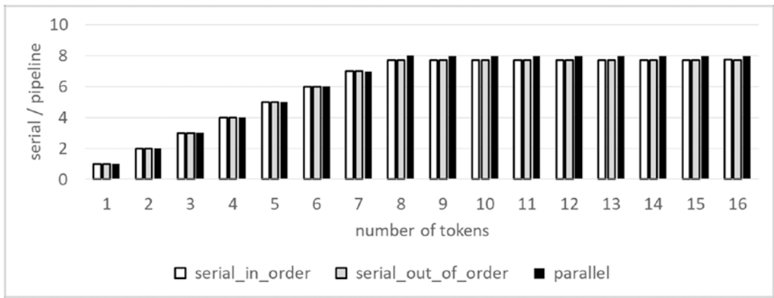
Figure 16-21. The speedup achieved by the different filter execution modes when executing a balanced pipeline with eight filters, 8000 items, and an increasing number of tokens. The filters spin for 100 microseconds.
