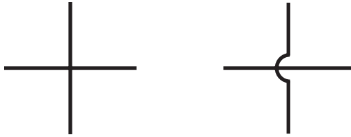
Figure 4-8: Nonconnecting crossed wires
