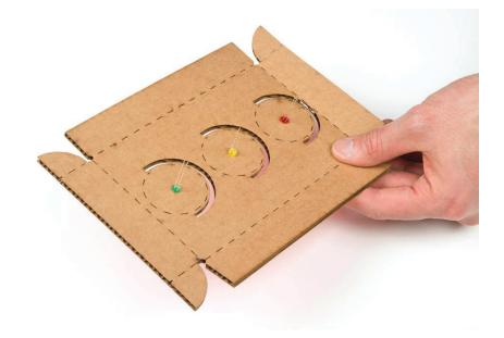
Next, bend the cardboard along the scored lines, as shown in Figure 2-19. Bend the vertical sides ① toward the interior, and then do the same with the top and bottom sides ② and the tabs ③. (The sides and tabs are labeled in Figure 2-15.)
