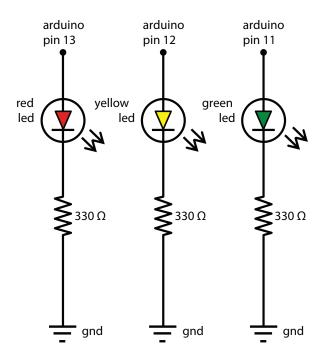
The schematic illustrates how each component is connected electrically. Pin 13, pin 12, and pin 11 on the Arduino will each be used to control an individual LED on the Stoplight circuit. As you can see in the schematic, each LED is connected to an individual resistor, and each resistor is connected to GND (ground). Next, let's look at the wiring.
