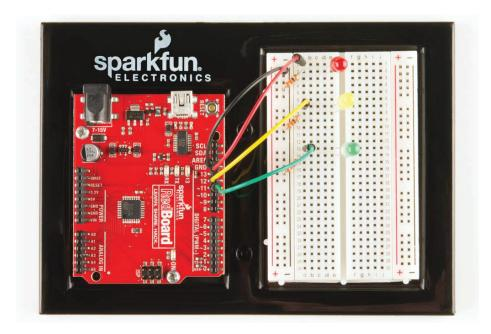
To mimic a real stoplight, this project needs a way to turn on each light for a certain amount of time and then switch to the next one. Fortunately, an Arduino sketch can use all kinds of instructions, including timing commands, to control a circuit.
