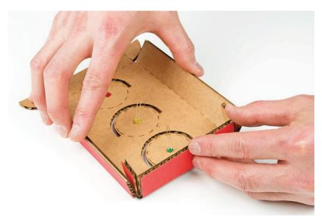
Position the tabs 3 inside the vertical sides 1, and glue them in place as shown in Figure 2-20. You can use hot glue, tape, or craft glue—we prefer hot glue because it's easy to work with, sets quickly, and has a pretty strong bond.
