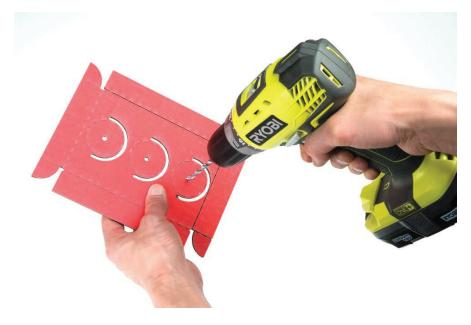
Once you have the holes drilled, remove the three LEDs from your breadboard and insert them through the back side of the cardboard, as shown in Figure 2-18. Remember that standard traffic lights are usually ordered red, yellow, and green from the top to the bottom. Pay attention to where the LEDs connect on the board, because we're going to reconnect them at the end.
