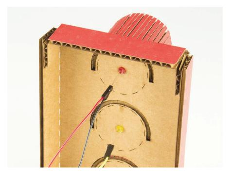
With the jumper wires connected to the LEDs, plug the male end into the breadboard in the same place where the LED came out, as shown in Figure 2-27. Again, pay attention to which LED goes where. If you don't remember, consult the original diagram in Figure 2-10.
