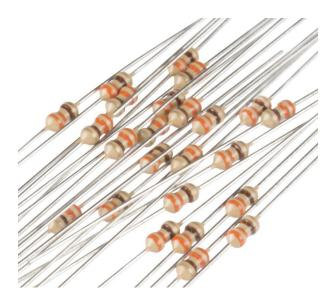
If you think of electricity like the flow of water through a pipe, a resistor is analogous to a point where the pipe size narrows, reducing the water flow. (If you're curious, see "Visualizing Electricity as Water in a Pipe" on page 4, which describes this metaphor in detail.)
