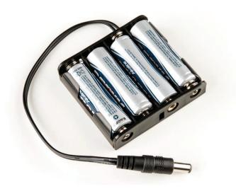
Unplug the USB cable from your computer, insert four AA batteries into your battery pack, and plug your portable battery pack into your Arduino, as shown in Figure 2-13. If your batteries are charged, you can move your project around or embed it directly into a model stoplight!
