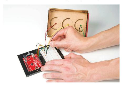
Check to make sure your connections work by plugging in the Arduino to your computer or to a battery pack. If one of the lights isn't working, try jiggling the connections or double-checking that the wires are plugged into the correct row on the breadboard.
