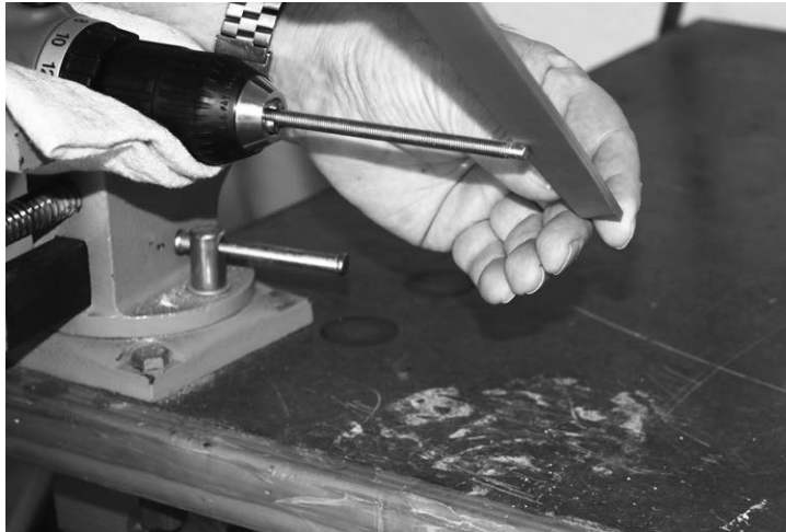
Figure 4-16: Reducing the diameter of the threaded shaft
