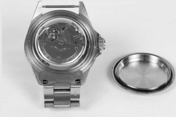
Figure 4-2: An automatic watch with the back removed, exposing the pendulum and the fulcrum (the screw in the center), which combine with a ratchet assembly to wind the watch's mainspring
