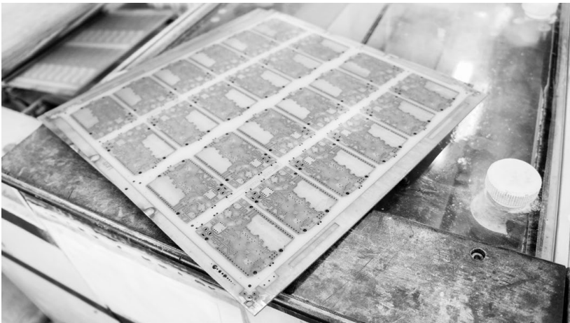
A panel etched of unwanted copper
