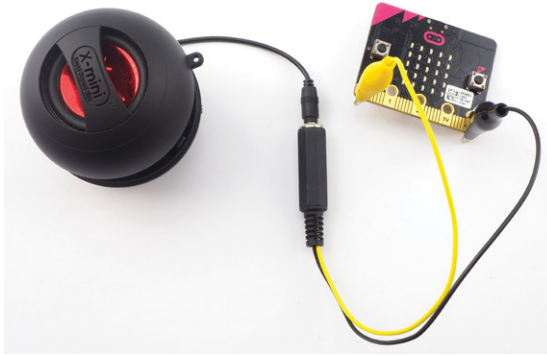
Figure 2-3: Connecting a micro:bit to an amplified speaker
