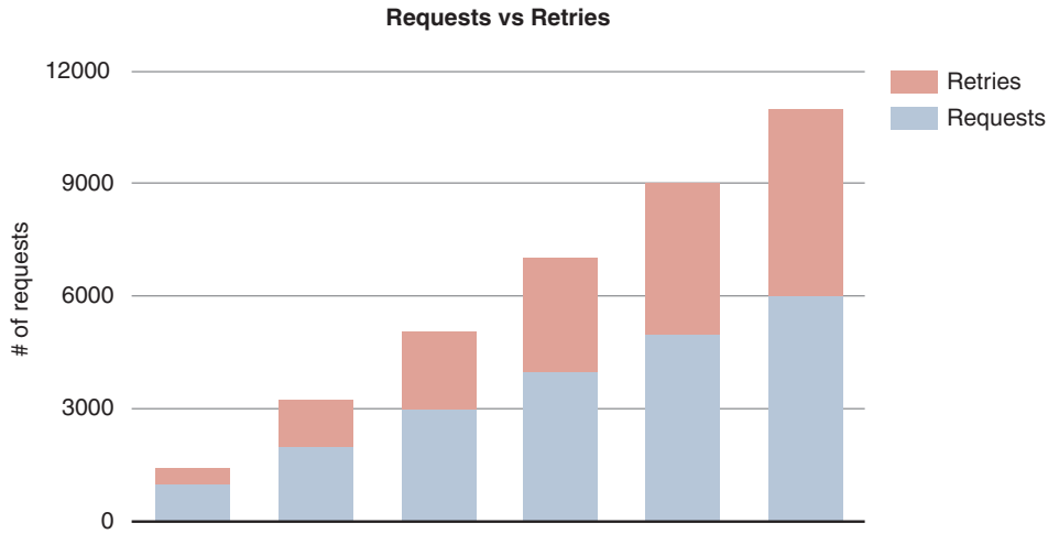
Figure 6.11 Growth of load on your unstable market-data service resulting from failed requests being retried
