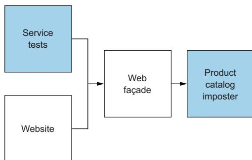
Figure 2.7 Virtualizing the product catalog service to test the web facade
