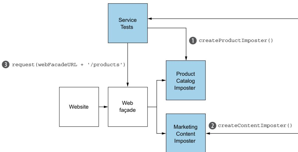
Figure 2.10 The steps of the service test to verify web façade's data aggregating
