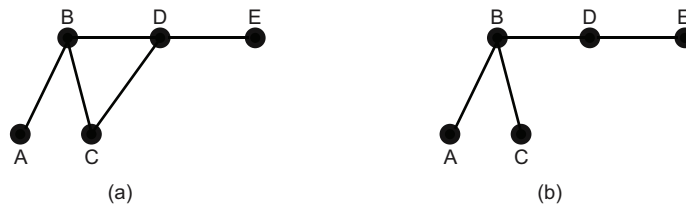
Figure 4.6 In (a), a cycle exists between vertices B, C, and D, so it is not a tree. In (b), the edge connecting C and D has been pruned, so the graph is a tree.
