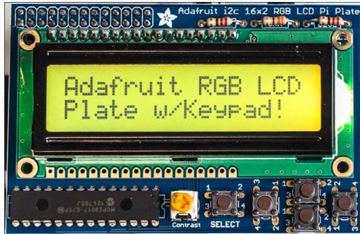
Adafruit I 2 C 16x2 RGB LCD Pi Plate with keypad buttons
