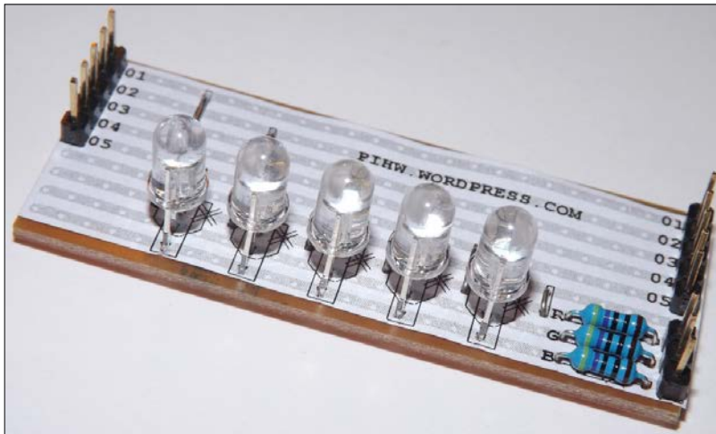
The RGB LED module from PiHardware.com
